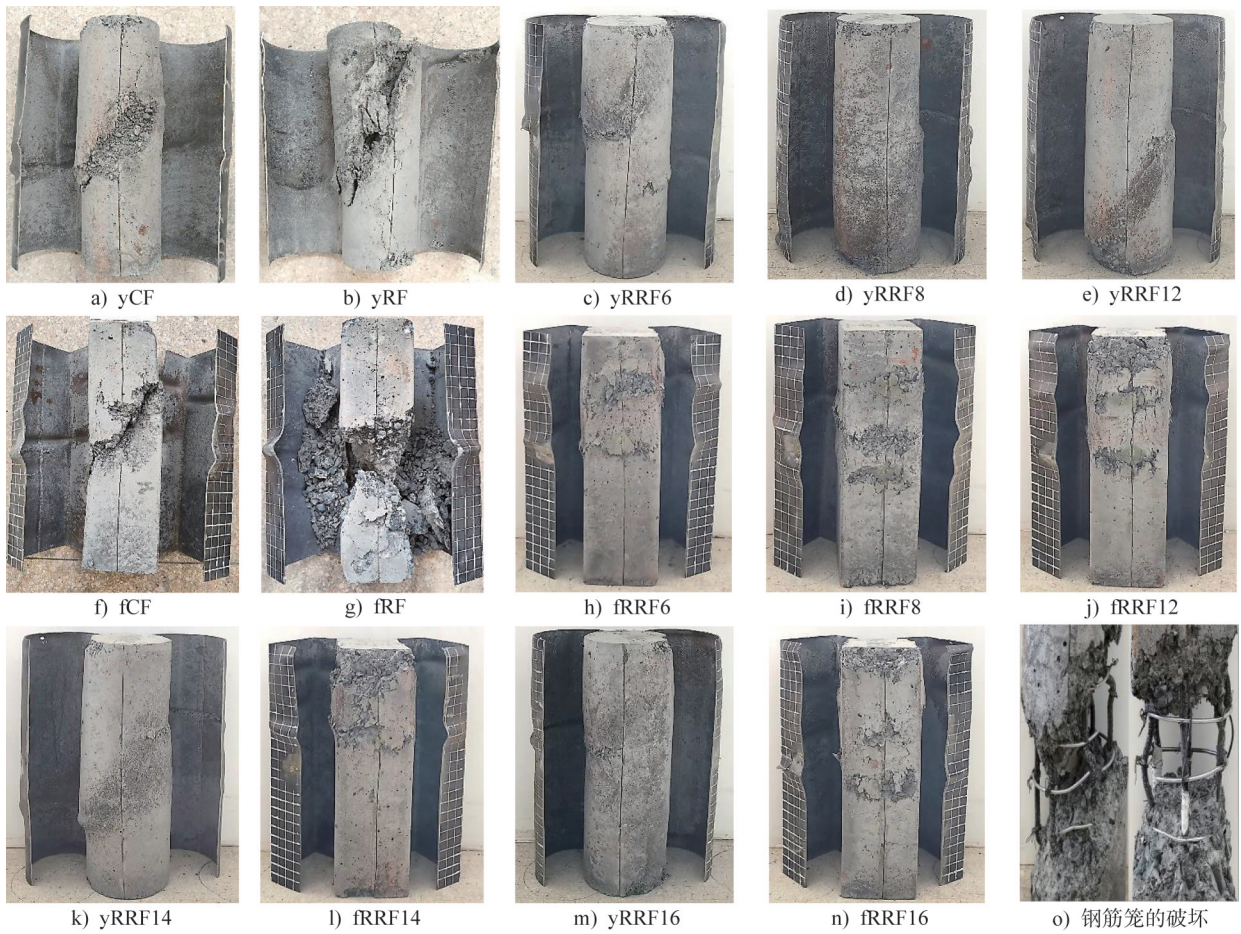
图4 各试件内部破坏形态 Fig. 4 Internal failure modes of specimens
