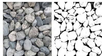
图 3 粗粒土照片图像处理 Fig. 3 Processing of images of coarse-grained soil samples
