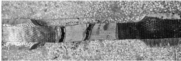
图4 单掺钢渣微粉试件开裂特征图 Fig.4 Cracking characteristics of single steel slag powder specimen
