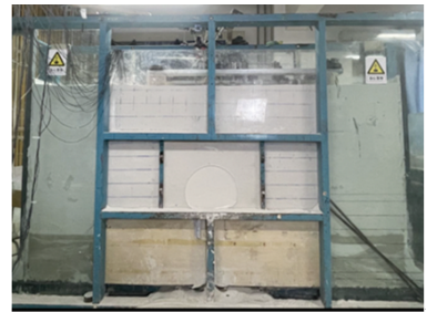
图 17 填土后模型架 Fig.17 Model test chamber after soil filling
