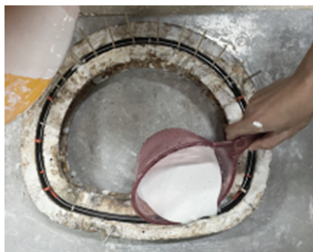
图12 石膏浇筑 Fig.12 Plaster casting
