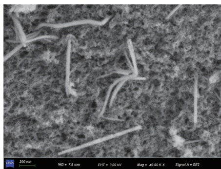
(c) Zr_{0.5}Ce_{0.5}O_2/NC SEM图
