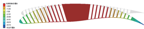
图 12 优化后的肋板垂直纵向位移云图 Fig. 12 Nephogram of the optimized floor vertical longitudinal displacement
