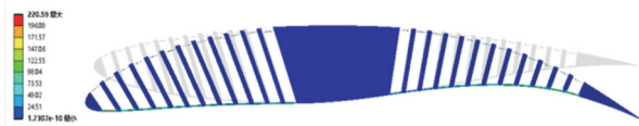
图 13 优化后的肋板等效应力云图 Fig. 13 Nephogram of the optimized floor equivalent stress
