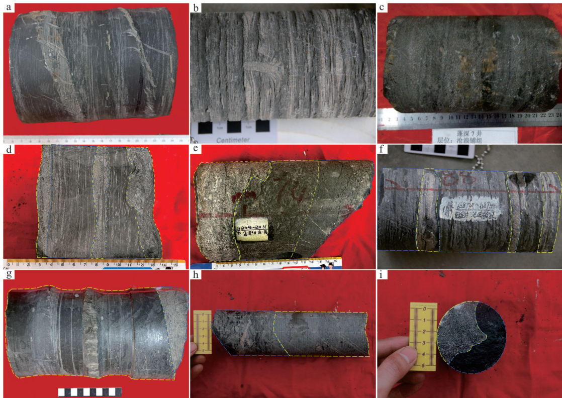
(a) 含白云质粉砂岩条带泥岩, PS2井, 7 274.20 m; (b) 条带状泥岩—含灰白云质粉砂岩, CT1井, 6 282.66~6 282.89 m; (c) 含泥质条带含砂灰质亮晶鲕粒白云岩, PS7井, 6 775.73~6 775.89 m; (d) 粉砂质泥岩与含砂质鲕粒白云岩互层, PS9井, 6 501.38~6 501.60 m; (e) 细粉晶白云岩—泥晶白云岩—含砂质鲕粒白云岩, PS9井, 6 510.34~6 510.51 m; (f) 含粉砂质灰质鲕粒白云岩—灰质粉砂质泥岩, CT1井, 6 287.30~6 287.45 m; (g) 粉砂质泥岩—细晶白云岩, PS2井, 7 275.85~7 276.09 m; (h) 含粉砂质灰质鲕粒白云岩—灰质粉砂质泥岩, PY1井, 6 903.36~6 903.58 m; (i) 含粉砂质灰质鲕粒白云岩—灰质粉砂质泥岩, PY1井, 6 903.71~6 903.81 m
