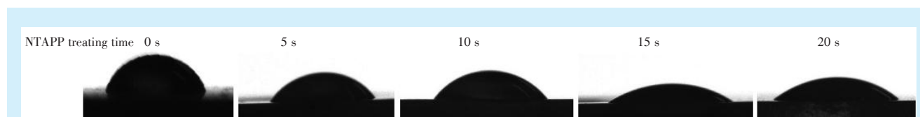
The contact angle of 0-15 s group decreased gradually, and the contact angle of 20 s group increased slightly. NTAPP: nonthermal atmospheric pressure plasma
