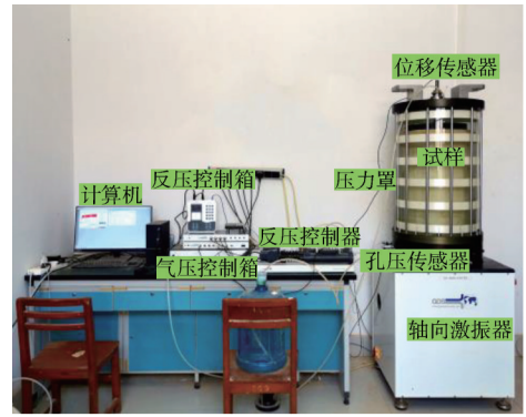
图1 DYNTTS大型三轴循环试验系统 Fig. 1 DYNTTS large triaxial cyclic test system
