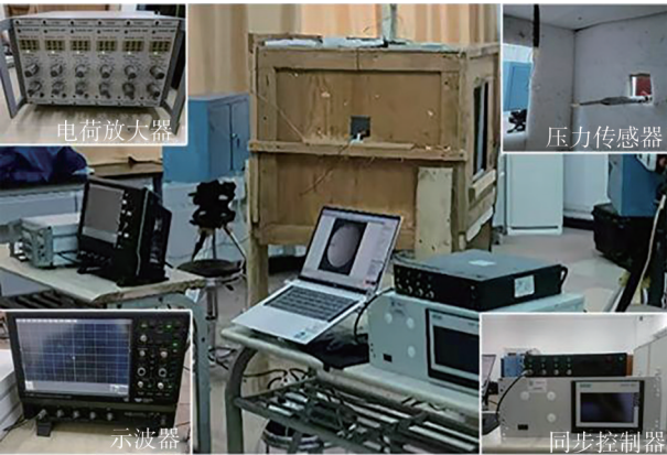
图 4 超压测试系统实物 [26] Fig. 4 Physical of overpressure test system [26]
