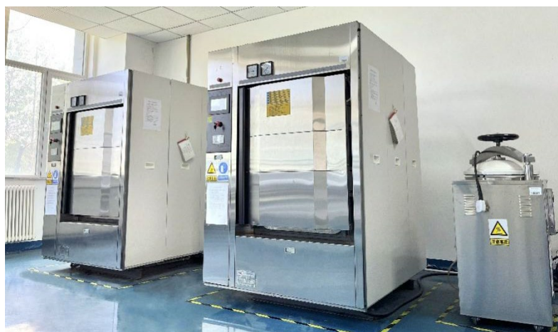
Fig. 4 Equip large pulsating vacuum sterilizers with warning signs, ground warning lines, operating procedures and usage records
